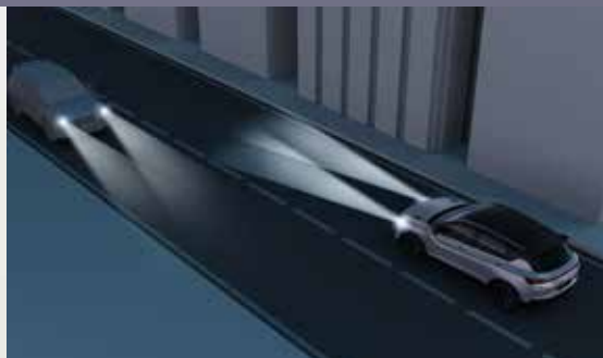
IHBC (Intelligent High Beam Control) system
