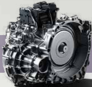
7-speed wet dual-clutch transmission
