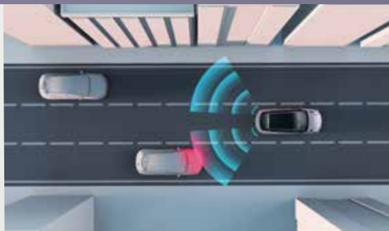
BSD (Blind Spot Detection) system
